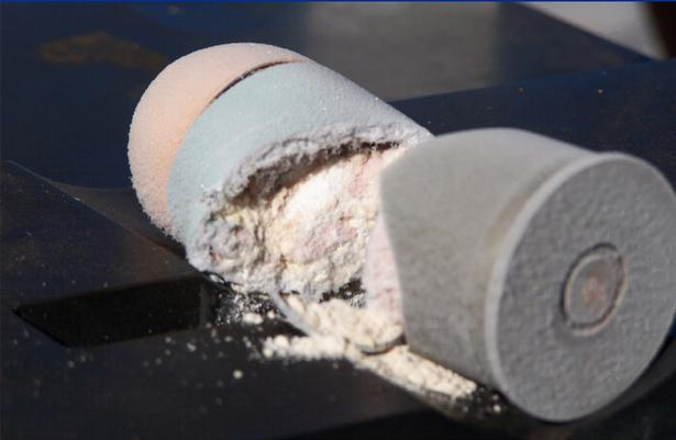
40mm HEPD grenade post cryofracture processing
