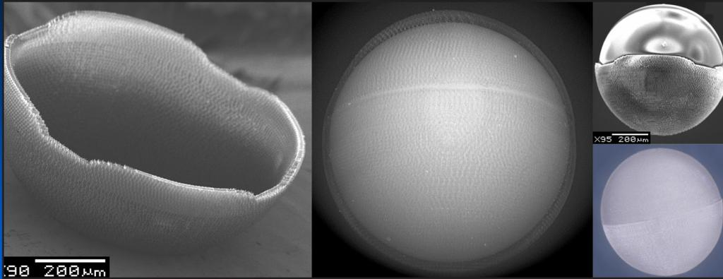
Thin-wall foam hemi mounted on direct-drive capsule
