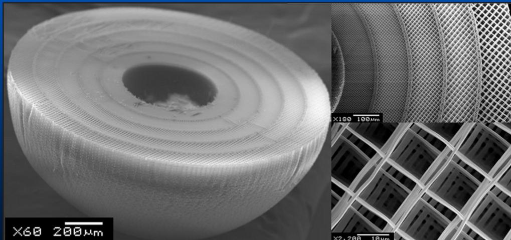
Gradient density foams in spherical geometries
