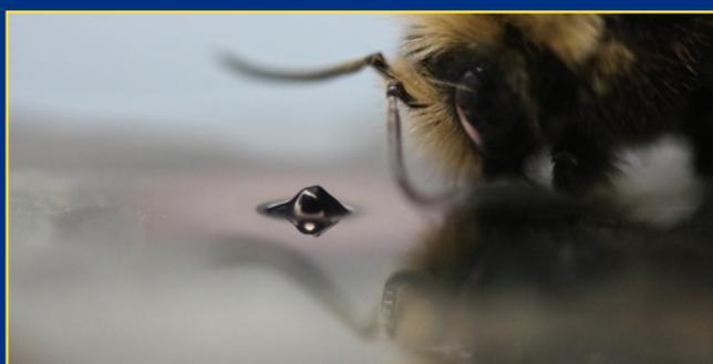
Sub-millimeter mound of copper aerogel applied with a nanoparticle deposition system next to a bee for scale
